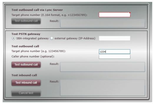
Image 3.26: Test of the Configuration via the web interface
