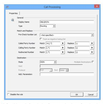
Image 3.62: Receiving calls from the interface, removing the prefix and routing to the Trunk
