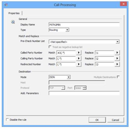
Image 3.60: Receiving calls from the first interface, removing prefix and routing to the PBX
