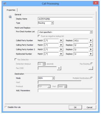
Image 3.58: Routing Trunk to ISDN
