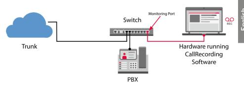
\* Please be advised that the use of an existent switch requires the configuration of a Monitoring Port. Should you utilize the Recording Bundle and the Managed Switch provided, port 8 will be the preconfigured monitoring port.
